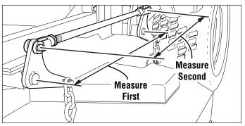
Figure 8. Check Lift Rod Timing
